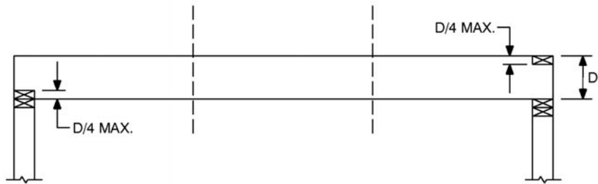
FLOOR JOIST—END CUTS
